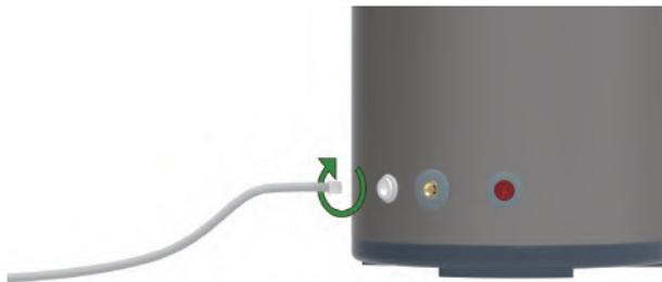
Fix the tube joint and fit the condensation tube to the overflow port. Finally, run it to suitable location.
