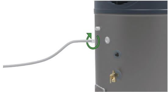
Fix the tube joint and fit the condensation tube to the overflow port. Finally, run it to suitable location.
