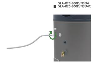
Fix the tube joint and fit the condensation tube to the overflow port. Finally, run it to suitable location.
