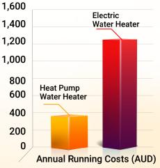
\*Estimations based on SLA-R25-300D-N4D4C in zone 3 under medium load, obtained from independent laboratory test results and followed by TRNSYS modelling and a retail electricity cost of \$0.30c per KWh.
